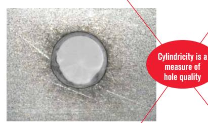
True Hole Technology requires a HyPerformance Plasma HPRXD auto gas system along with a True Hole enabled cutting table, nesting software, CNC, and torch height control. Consult with your table manufacturer for more details.
